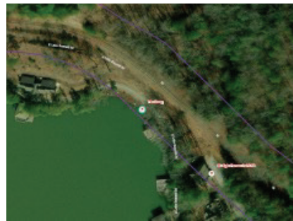
Floodway Encroaches in Rail Corridor (35.23, -82.41) 100-year floodplain encroaches into rail corridor.
