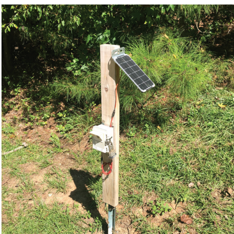
A trail counter at the Pump Station access at Eno River State Park
