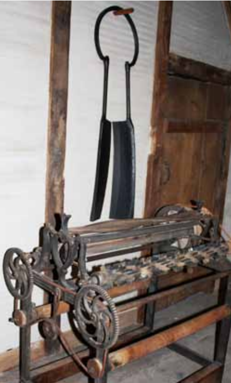
Large, heavy shears (on the wall) used to cut the nap on woolen fabrics were replaced by machines with a helical blade in the 19th century.
