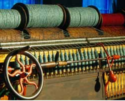
Spinning jack, c. 1864. Men who operated spinning jacks were highly skilled, and often the highest-paid employee in a mill.
