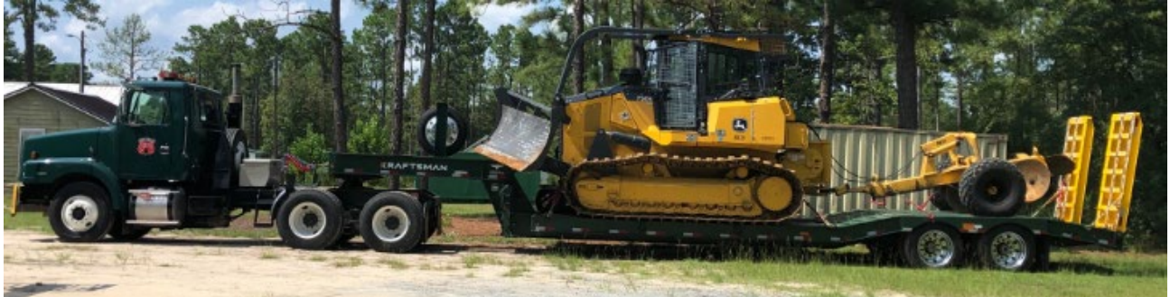
Figure 8. This John Deere 750K is one of the 92 wildland fire tractor plow units across the state.
